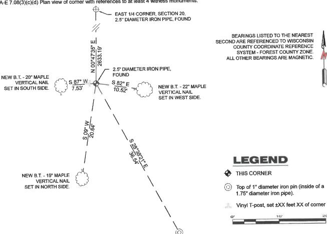
A-E 7.08(3)(e) 1865 Surveyor set a post, 1985 Surveyor found a 1 1/4" iron pipe, 2002 Surveyor found a 2" pipe. I found a 2.5" outside diameter iron pipe.
