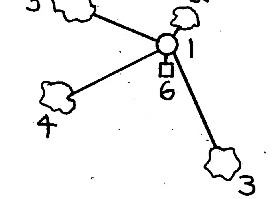
Describe any material discrepancy between the location of the corner as restored or reestablished and the location of that corner as previously restored or reestablished by distance and direction. Show the discrepancy on the plan view drawing under (d), above. Show the distances between the corner as previously restored or reestablished and (1) the corner as restored or reestablished, and (2) to at least 2 of the witness monuments shown on the drawing in (d), above.
