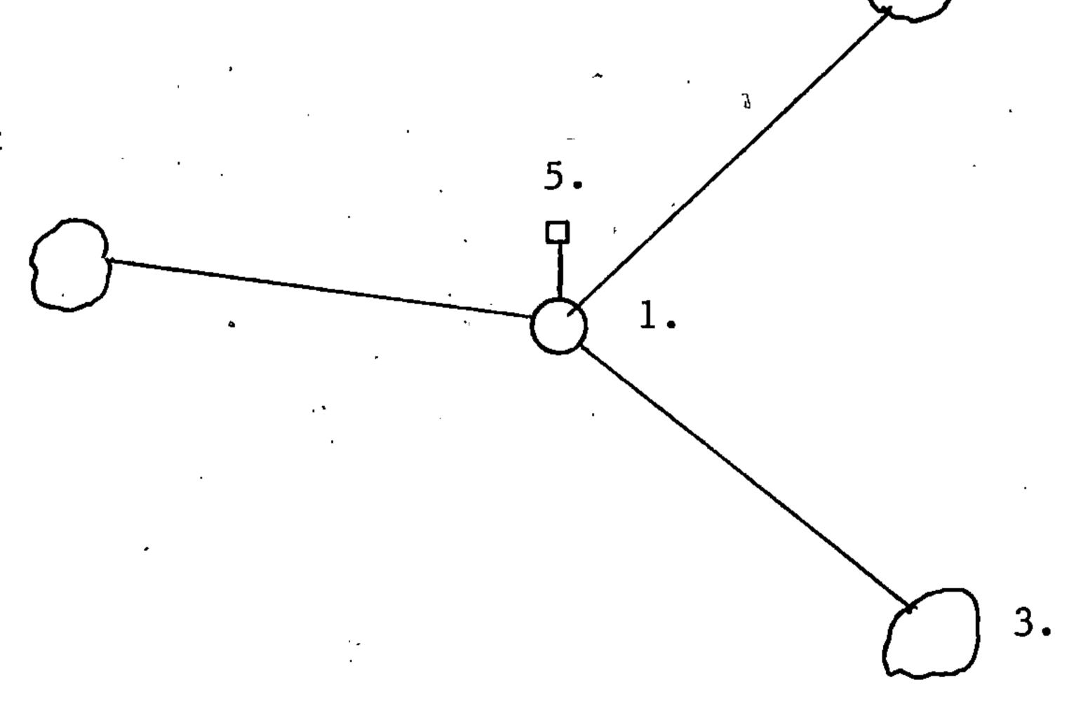
(a) Describe any material discrepancy between the location of the corner as restored or reestablished and the location of that corner as previously restored or reestablished by distance and direction. Show the discrepancy on the plan view drawing under (d), above. Show the distances between the corner as previously restored or reestablished and (1) the corner as restored or reestablished, and (2) to at least 2 of the witness monuments shown on the drawing in (d), above.
