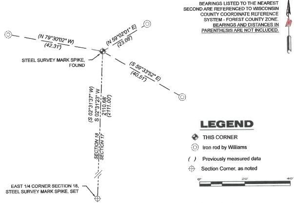
A-E 7.08(3)(e) 2019 Surveyor set a 1" x 4" survey spoke. I found a steel survey mark spike with a 1" diameter head.
