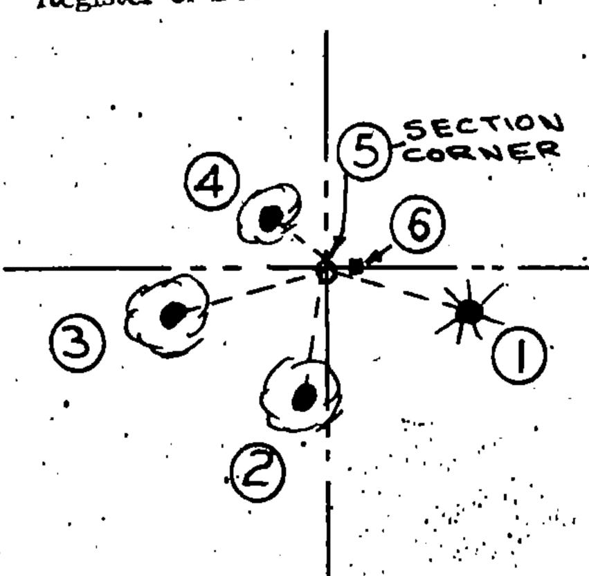
(e) Describe any material discrepancy between the location of the corner as restored or reastablished and the location of that corner as previously restored or reastablished by distance and direction. Show the discrepancy on the plan view drawing under (d), above. Show the distances between the corner as previously restored or reastablished and (1) the corner as restored or reastablished, and (2) to at least 2 of the witness monuments shown on the drawing in (d), above.
