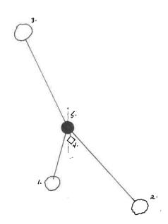
(e) Describe any material discrepancy between the location of the corner as restored or reestablished and the location of that corner as previously restored or reestablished by distance and direction. Show the discrepancy on the plan view drawing under (d), above. Show the distances between the corner as previously restored or reestablished and (1) the corner as restored or reestablished, and (2) to at least 2 of the witness monuments shown on the drawing in (d), above.
