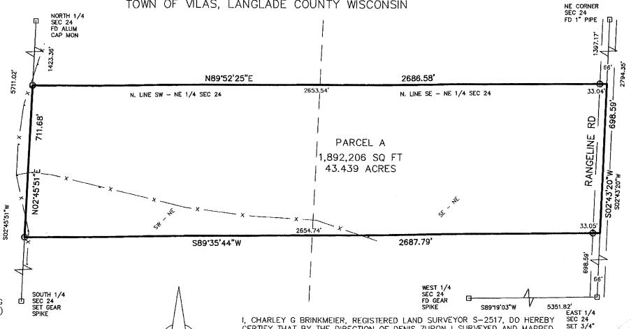
O 1.3" X 18" IRON PIPE WEIGHING 1.68 LBS/LINEAL FOOT SET(OD)
