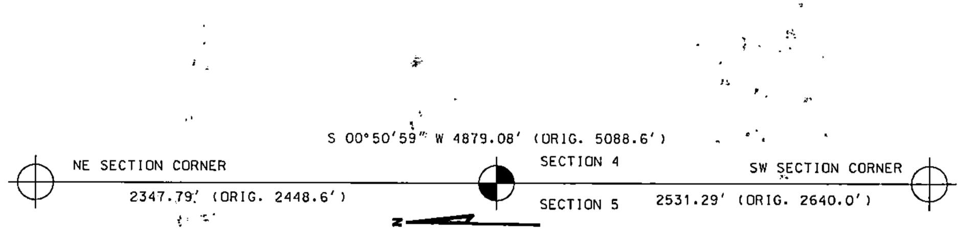
(c)(d)(e) Plan view of corner with ties to at least 4 witness monuments. If in disagreement with previously established corner, show the distances between the two corners and also indicate the ties to the
