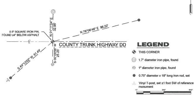
A-E 7.08(3)(e) 1865 Surveyor set a post, 1964 Surveyor set a galvanized iron pipe with an aluminum Kimberty Clark cap, 1993 Surveyor found a nail and a witness corner. 2023 - I found a 0.5" square iron pin.
