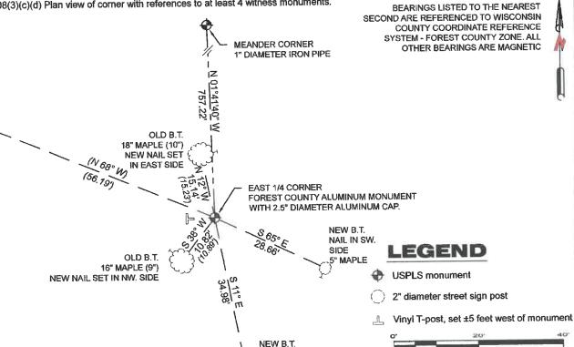
A-E 7.08(3)(e) 1865 Surveyor set a post, 1995 Surveyor found a 1" diameter iron pipe and replaced it with a "standard Forest County aluminum monument, subsequent surveyors found aluminum monuments of varying sizes. I found a Forest County aluminum monument with a 2.5" diameter cap stamped to identify corner. SCONS/
