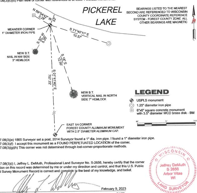
A-E 7.08(3)(e) 1865 Surveyor set a post, 2014 Surveyor found a 1" dia. iron pipe. I found a 1" diameter iron pipe.
