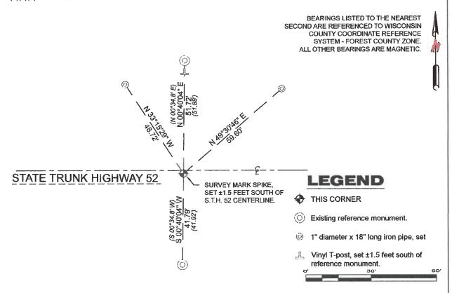
A-E 7.08(3)(e) 1857 Surveyor set a post, 1985 Surveyor set a railroad spike. 2023 I set a steel Survey Mark spike.
