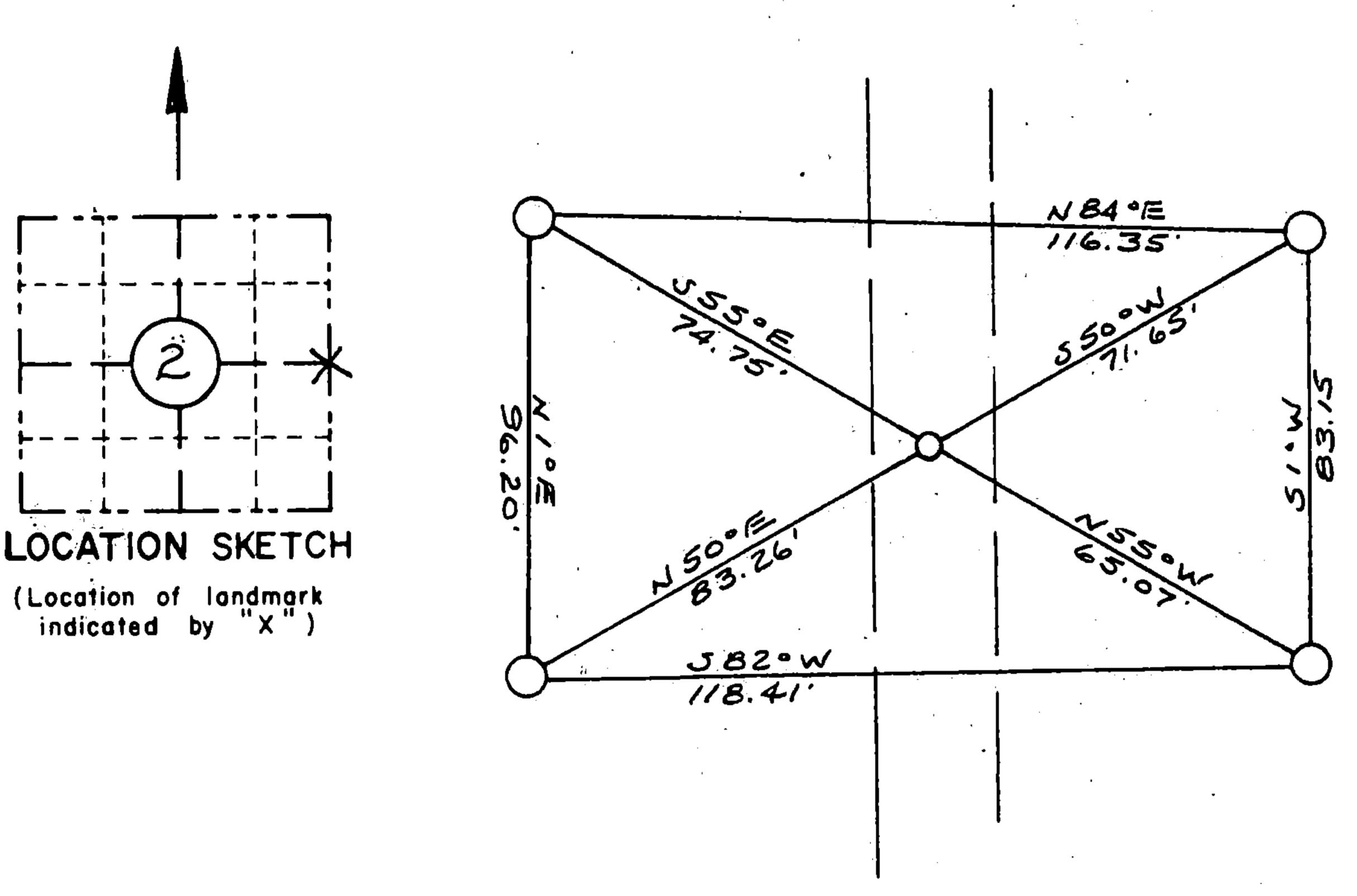
I hereby certify that on the Am day of MAY 1993, that I did locate the above corner which was evidenced by R.R. SPIKE ; I further certify that to perpetuate the location of such corner I did, at the exact location thereof, place a permanent marker consisting of NONE ; I further certify that I did establish 4 references or witness monuments consisting OF 5/8" X 24" RE-BARD WITH RED PLASTIC SEAL WDOT CAPS located as shown above:
