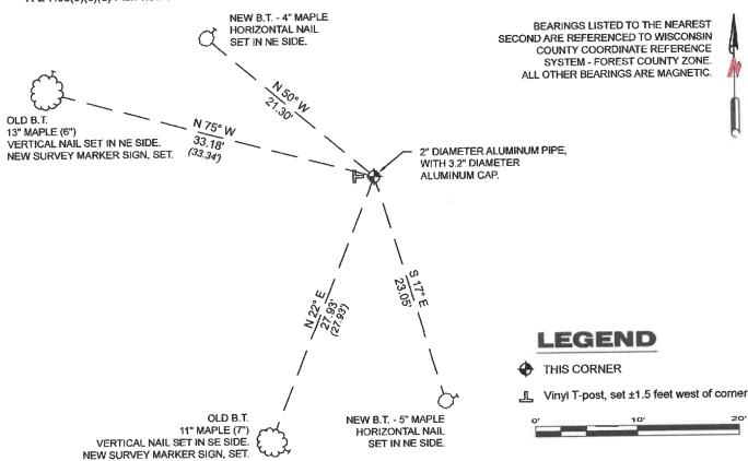
A-E 7.08(3)(e) 1859 Surveyor set a post, 1977 Surveyor set a 2 1/2" Berntsen, A-1 Federal monument, 2009 Surveyor found a 2" alum. pipe mon.. 2023, I found a 2" diameter aluminum pipe, with a 3.2" diameter aluminum cap, stamped to identify corner.
