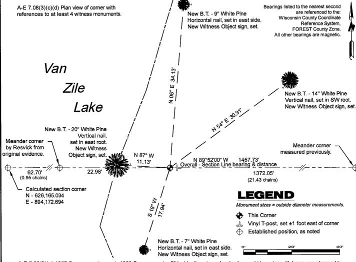
A-E 7.08(3)(e) 1857 Surveyor set a post, 1969 Surveyor set a 2" inside diameter galvanized wrought iron pipe with brass cap stamped to identify corner. I set an aluminum pipe monument in 2025.
