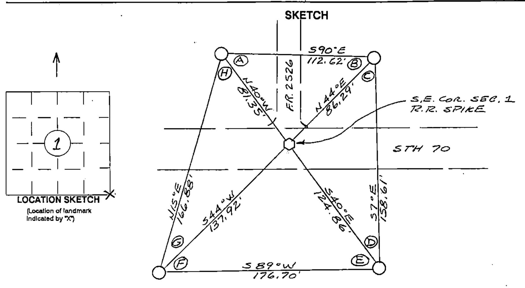
ANGLE TABLE  $A = 49^{\circ} 40' 58''$   $B = 45^{\circ} 57' 53''$   $C = 51^{\circ} 34' 31''$   $D = 32^{\circ} 46' 38''$   $E = 50^{\circ} 57' 49''$   $F = 44^{\circ} 41' 03''$   $G = 29^{\circ} 01' 16''$  H = 55'' 19' 52''
