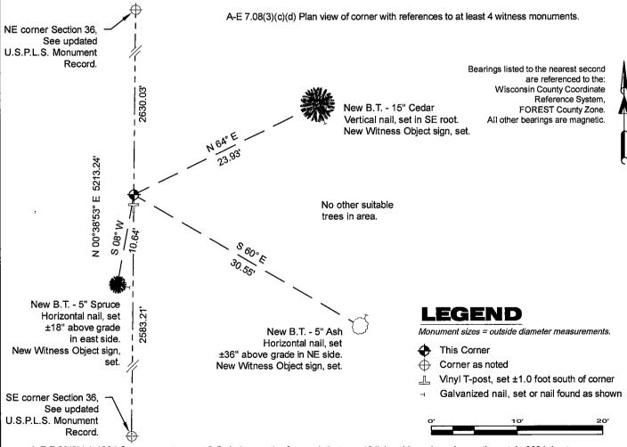
A-E 7.08(3)(e) 1864 Surveyor set a post 3.5 chains north of a creek that was 10 links wide and running north east. In 2024, I set a 1" diameter X 32.5" long drivable, Forest County aluminum pipe with a 3.25" diameter aluminum cap stamped to identify the corner, 231" north of a creek with the same description.
