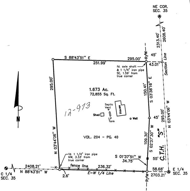
Bearings are referenced to the East Line of the NE 1/4 of Section 35, assumed to bear N 03'44'06" W.
