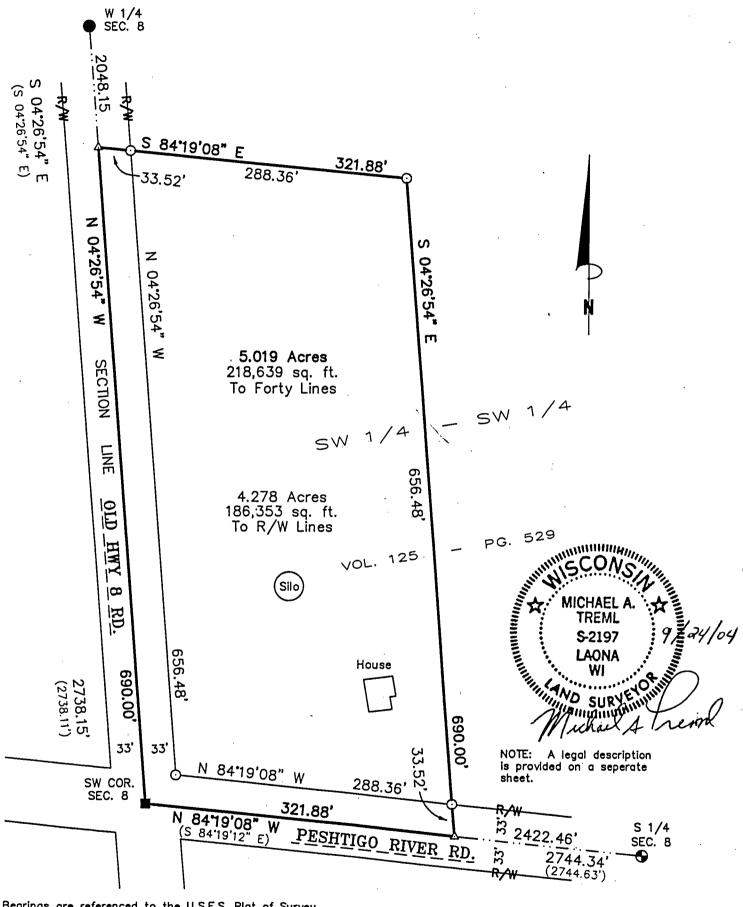
Bearings are referenced to the U.S.F.S. Plat of Survey, the West Boudary Line of the SW 1/4 of Section 8, Bears S 04°26'54" E.
