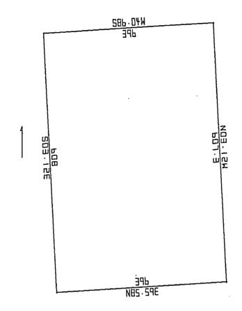
Masler | ...... AREA ...... | .. CLOSING ERROR .. Scale : 156 ft/in | Acres : 5.524 | Bearing: N00.2332E North Shift: +0 | Sq. Feet : 240607 | Feet : 0.12 East Shift : +0 | Sq. Meters: 22353.1 | Meters : 0.04 DMS Rotated: +000.0000 | Perimeter : 2007.30 | Precision: 1/16144
