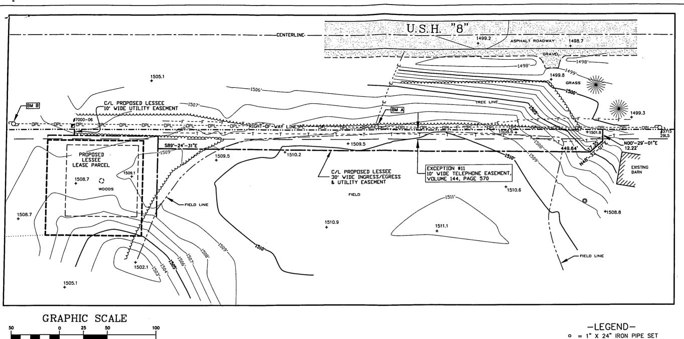
BEARINGS REFERENCED TO THE WISCONSIN STATE PLANE COORDINATE SYSTEM (NAD83/91) — NORTH ZONE
