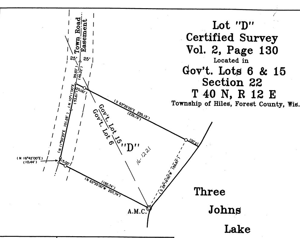
FOREST CO SURVEYOR FILE # 401222-2006 0414 BEARINGS ARE ALL TAKEN FROM THE RECORDED CERTIFIED SURVEY MAP, VOL. 2, PAGE 130. THE PURPOSE OF THIS SURVEY WAS TO MARK THE 15 FOOT SIDELINE SETBACKS AND THE 75 FOOT LAKE SETBACK FOR BULDING PURPOSES.
