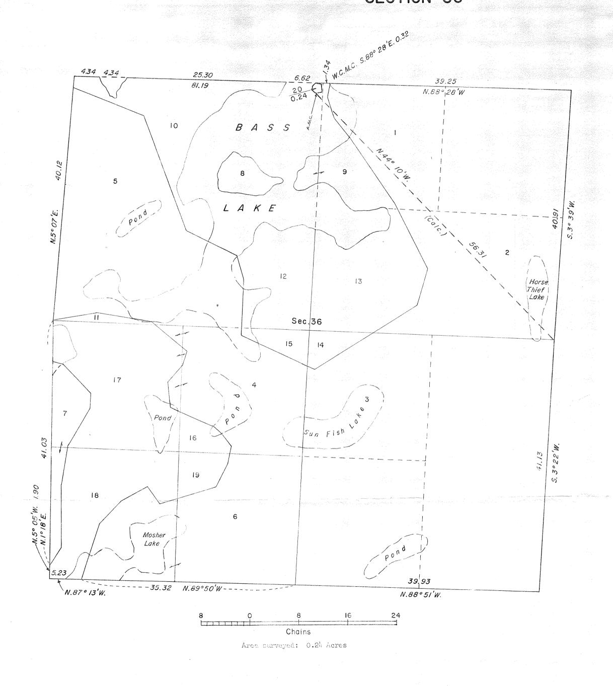
This supplemental plat of section 36, giving area and designation to an island in Bass Lake not previously shown on an official plat, is based entirely on the record of an island survey in section 36 by C. M. Pidgeon, U. S. Surveyor, in 1911, and a dependent resurvey and extension survey in section 36 by A. W. Brown, U. S. Cadastral Engineer, in 1931.
