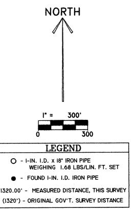
BEARINGS AND COORDINATES ARE BASED ON THE LANGLADE COUNTY COORDINATE SYSTEM, NAD 1983 (91) DATUM, AND ARE REFERENCED TO THE NORTH LINE OF THE NORTHWEST 1/4 OF SEC. 4, T32N, RIOE, MEASURED TO BEAR N89°13'48"E. CCORDINATES AT THE SOUTH 1/4 CORNER OF SEC. 4, T32N, RIOE, OF N.390381.2794/E.594625.6325 WERE PROVIDED BY THE LANGLADE COUNTY SURVEYOR'S OFFICE AND HELD AS A COORDINATE BASE POINT FOR THIS SURVEY.
